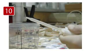
Pull gently on the trigger until the resin is ejected from the end of the static mixer. Make sure that the cartridge is inclined as shown in the image.
