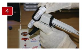
Making sure the plunger is all the way home, lift the flap and place the cartridge into the dispensing gun.
