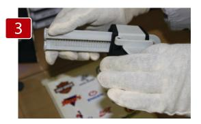
Place plunger into dispenser, ensuring serrated edge faces the handle - making sure the plunger is all the way home.
