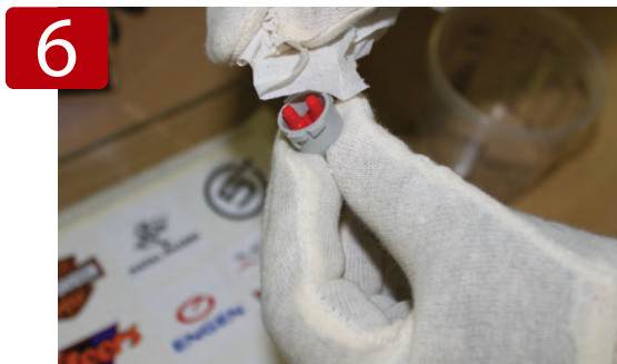
Be sure to wipe the night cap, once removed, to avoid complications later when resealing.
