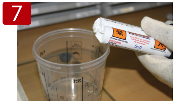
Squeeze the dispenser until both cylinders are ejecting resin. Make sure the cartridge is inclined as show in the image. (Back lower than dispensing tubes).
