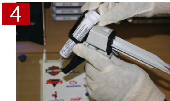
Making sure the plunger is all the way home, lift the flap and place the cartridge into the dispensing gun.
