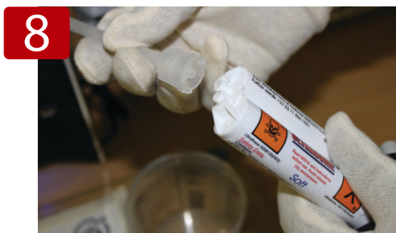
Now attach the static mixer to the cartridge. Aligning the tubes on the cartridge, gently push them together.
