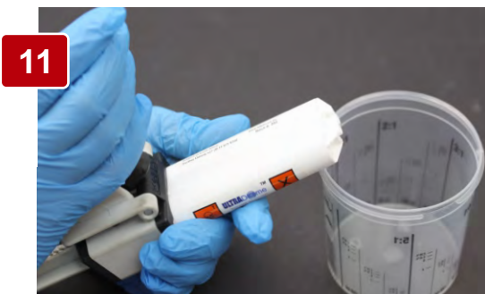
11 Purge cylinders until resin exits from both openings, inclining gun lower than receptacle.
