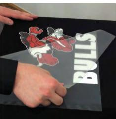
Maizey's heat presses are engineered to permanently imprint designs or graphics produced on heat transfer materials on fabric substrates with the application of heat and pressure. Our heat presses provide adjustable pressure settings, uniform heat distribution across the surface of the heating plate and accurate timing controls, ensuring perfect application.
