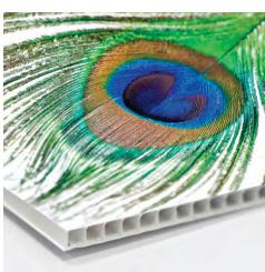
An extruded, fluted polypropylene board, (similar to corrugated cardboard) that is environmentally friendly, waterproof and recyclable. Coruplas has very good stiffness due to the twinwalled, fluted surface and provides a cost effective option for indoor and short term outdoor signs.
